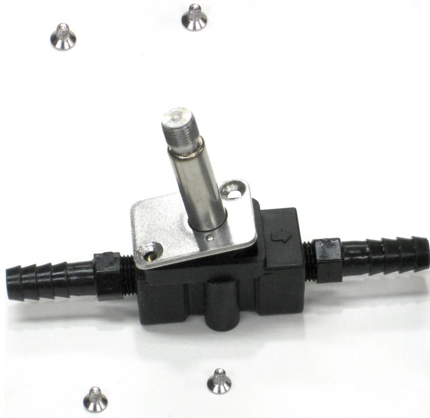
Place the plunger into the body, the pad end goes in first, then position the stem and retainer plate over it. Align the screw holes and insert the screws. Tighten the screws but do not over tighten them.
