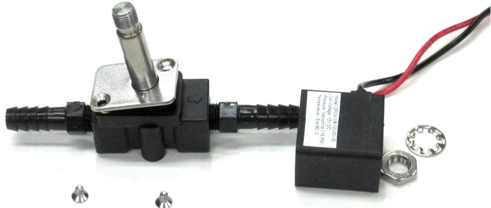
The stem and retaining plate should popup, If they don't then gently work the stem by rocking it side to side. Do not use a lot of force as there is an "O" ring that can be damaged.
